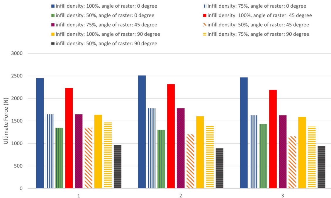
Figure 11. Maximum force applied in tensile loading on carbon fibers reinforced PLA.
