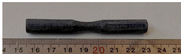
Figure 7. 3D printed carbon fibers reinforced PLA fatigue specimen. Photo was taken by the authors.
