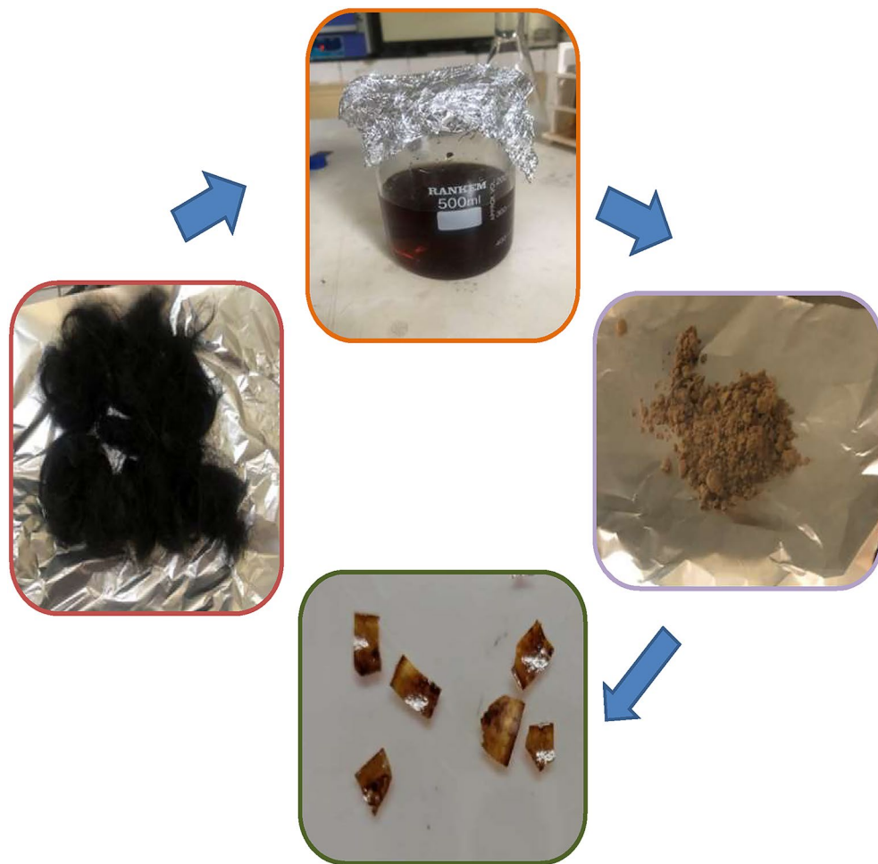
Figure 1. Overview of bioplastic production. Clean hair samples were delipidized in chloroform and methanol followed by the incubation with extraction buffer to extract keratin. Extraction buffer composed of urea, thiourea, betamercaptoethanol and tris-HCl. The obtained protein extract was dialyzed and lyophilized to obtain the protein powder which was further utilized to obtain bioplastic film by solution casting with various plasticizers. See text for details.
