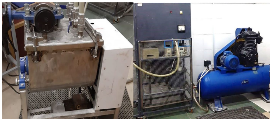
Figure 3. Laboratory ion–ozone cavitation unit for accelerated dough preparation.
