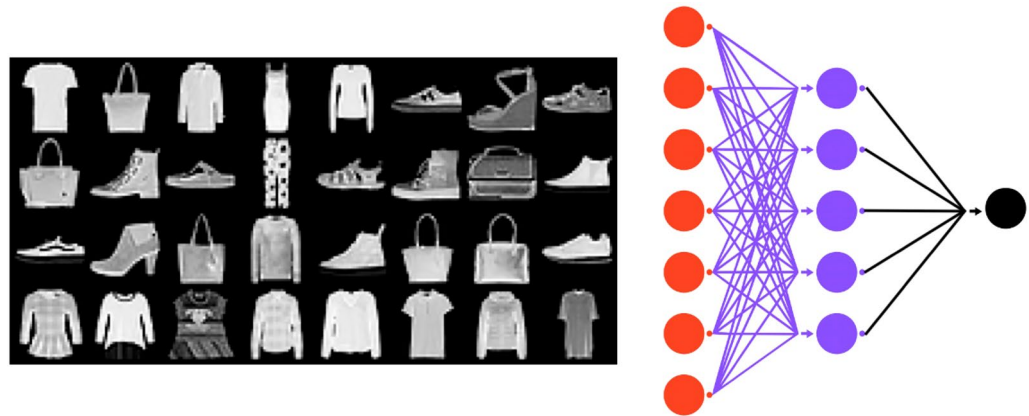
Figure 7. Phase transition analysis for the DNN architecture training using the Fashion MNIST dataset. Data samples are 28 \times 28 pixel images from the 10 classes of the Fashion-MNIST dataset using a NN architecture of 784-32-10 input-hidden-output neurons.
