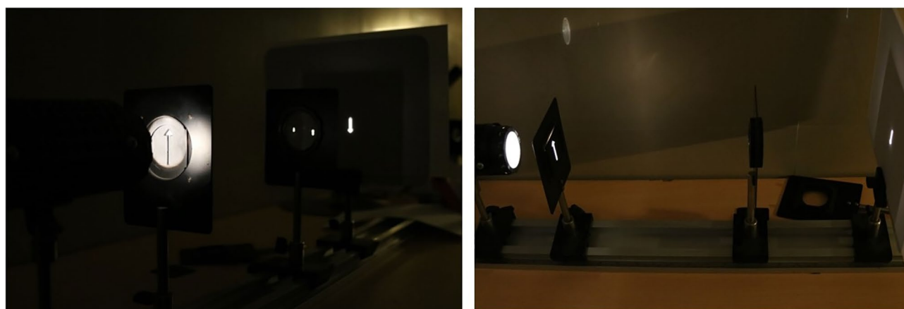
Figure 1. Image formation by convex lens: The image of an arrow is formed by a positive lens on the observation screen. By changing the distance of the object, residents can see the place of image formation and the magnification changes. Also, by moving the lens vertically, the image moves and the prismatic effect of the lens can be observed. In addition, with this experiment, depth of field and depth of focus can be measured.
