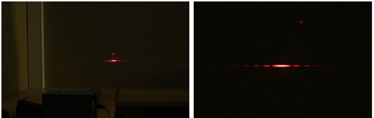
Figure 2. Single-slit diffraction pattern. In this experiment, the Wave nature of light can be shown. As the width of the slit producing a single-slit diffraction pattern is reduced, the diffraction pattern becomes wider and vice versa.
