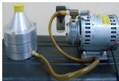
Figure 2. Two-stage Andersen sampler.
