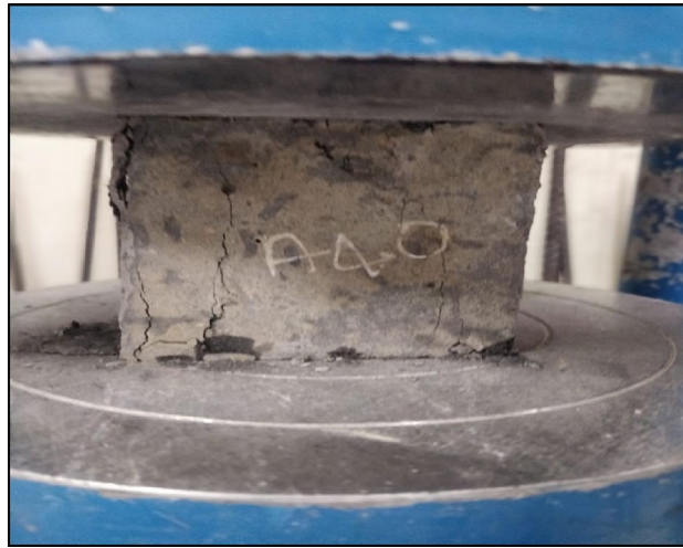
Figure 8. Failure of WPCB fibre-reinforced cube under compression.
