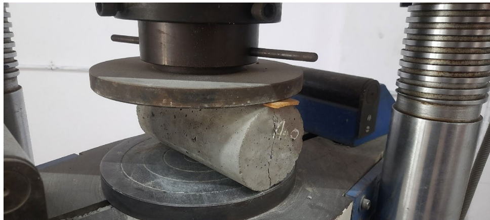
Figure 11. Failure of WPCB fibre-reinforced cylinder under split tension.
