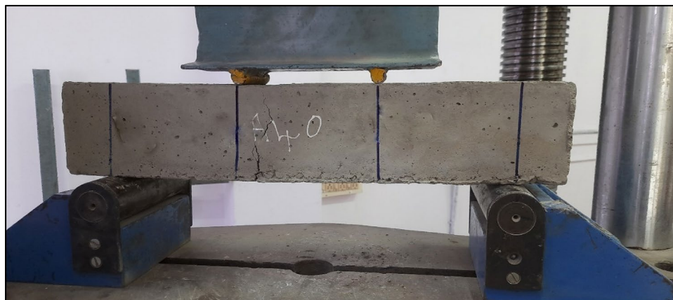
Figure 14. Failure of WPCB fibre-reinforced prism under flexure.
