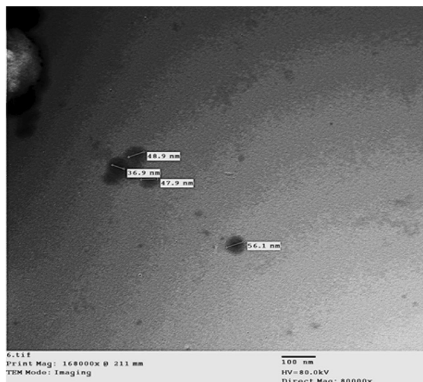
Figure 3. TEM micrograph of spherical shaped synthesized SeNPs performed at 10 mM sodium selenate, 1.5% ascorbic acid and coated with gum Arabic ( \approx 46.9 nm, including coat).
