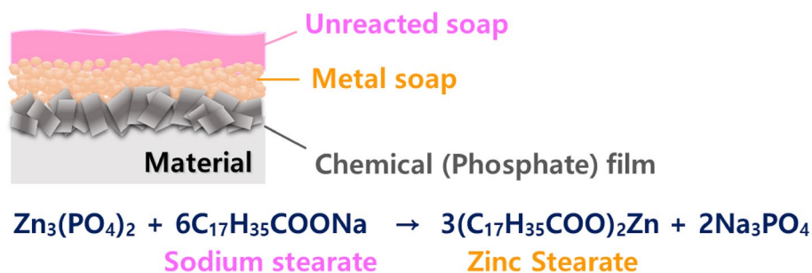
Figure 2. Structure of phosphate lubrication system.
