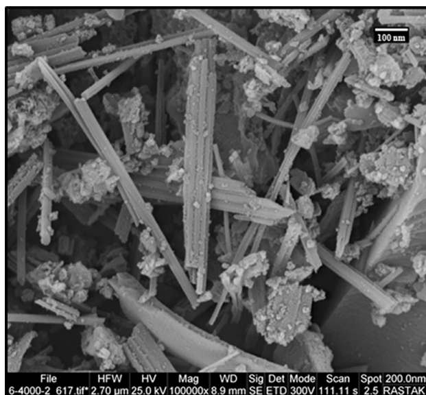
Figure 10. SEM images of recovered RL BF Fe-based MOF@CuO NC.
