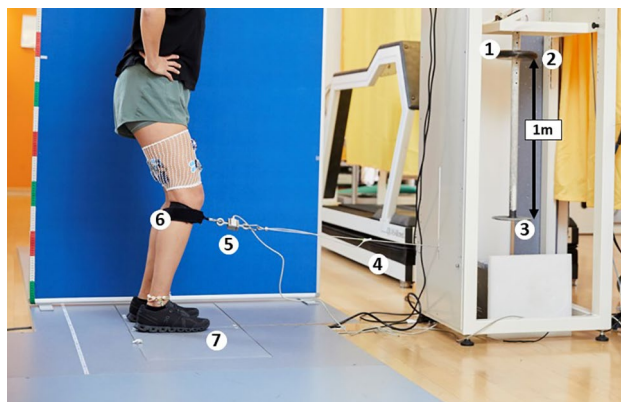
Figure 3. Stretch reflex measurements in upright standing position (©BFH Bern Movement Lab). (1) Electromagnet, (2) falling barbell weight, (3) stopper, (4) wire rope, (5) force transducer, (6) brace, (7) two force plates.
