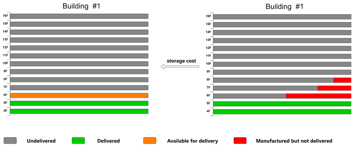
Figure 4. Unfinished production of target layer components.
