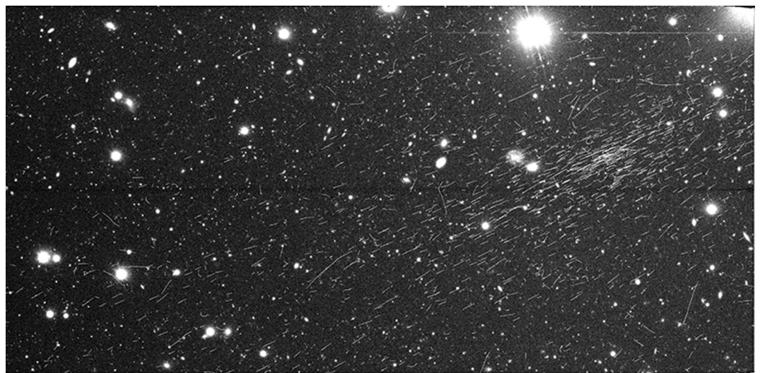
Figure 1. An example of a cosmic-ray extensive air shower recorded by a CCD of Subaru HSC. Dimensions: 4176 × 2048 pixels = 62.6 mm × 30.7 mm. The high density of aligned tracks, indicative of an EAS, is clearly visible in the upper right portion of the image.
