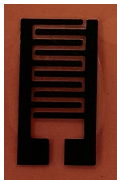
Figure 8. A digital photograph of LIG electrode pattern on Kapton paper.
