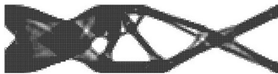
Figure 15. Design obtained using standard HCA algorithm without similarity constraints for the 2D crash TO problem.
