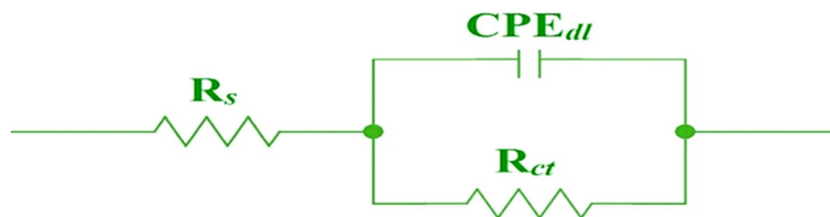
Figure 10. Equivalent circuit used for fitting EIS graphs.
