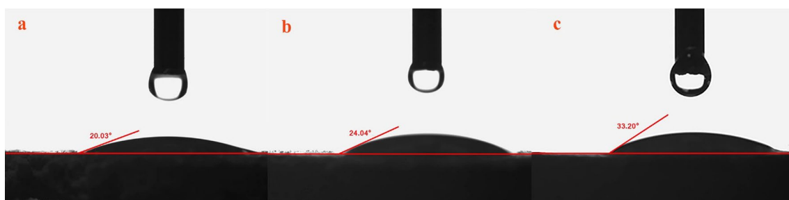
Figure 11. The contact angle measurement of (a) Mt; (b) Mt + PAA-DMAPS; (c) Mt + PAA-DMAPS-AMPS.
