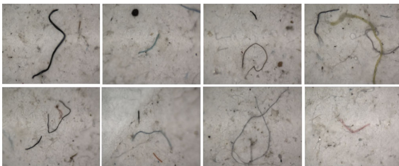
Figure 6. Optical images of different microfibers extracted from the laundry wastewater.
