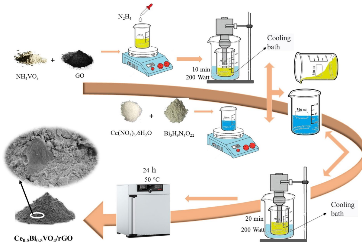
Figure 1. Synthesis steps of \text{Ce}_{0.5}\text{Bi}_{0.5}\text{VO}_4/\text{rGO} nanocomposite.
