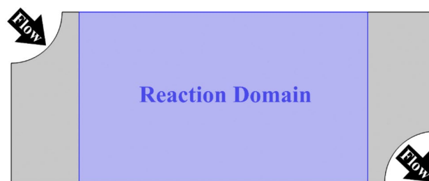
Figure 9. Microreactor design domain, \Omega . The reaction domain, \Omega_r , is highlighted in blue. The inlet is located at the top left corner and the outlet is located at the bottom right corner.
