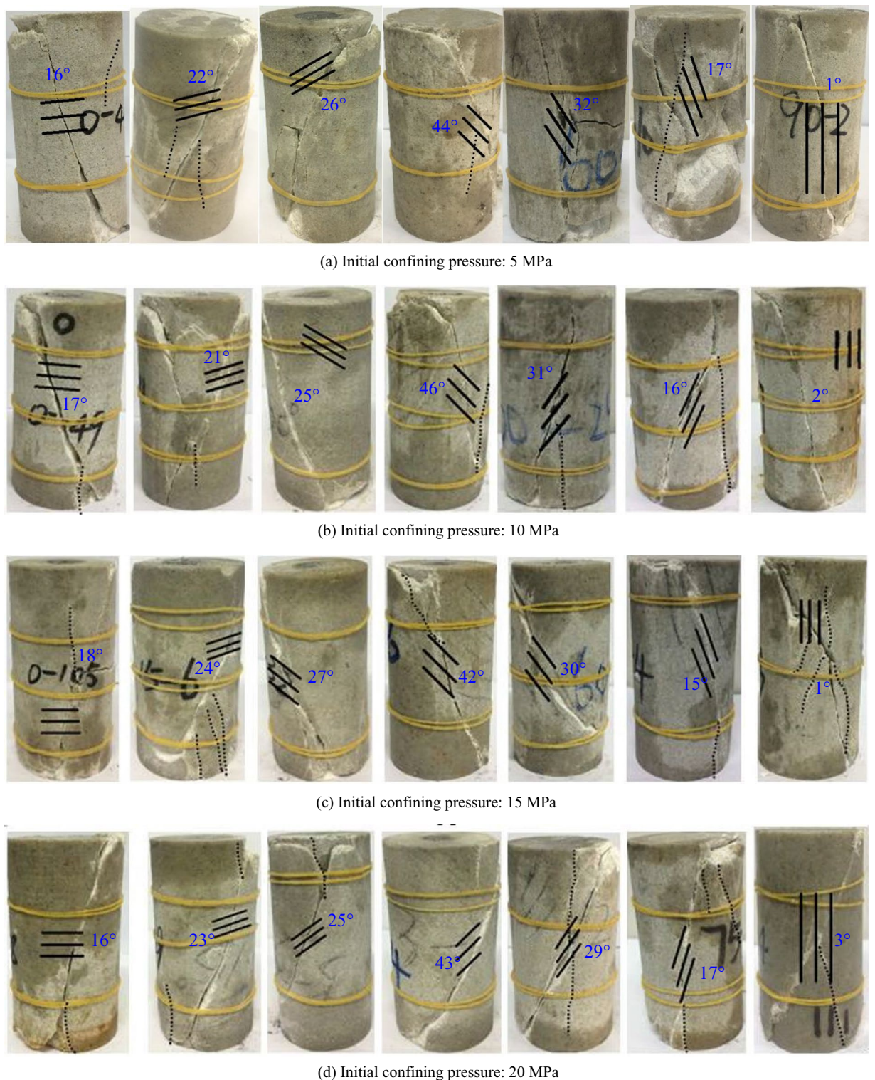
Figure 12. Typical cracked rock specimens.
