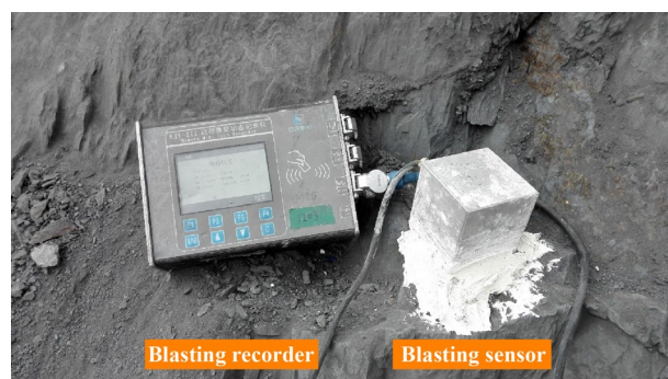
Figure 10. The monitoring of blasting vibration on the groundwater-sealed tunnel.
