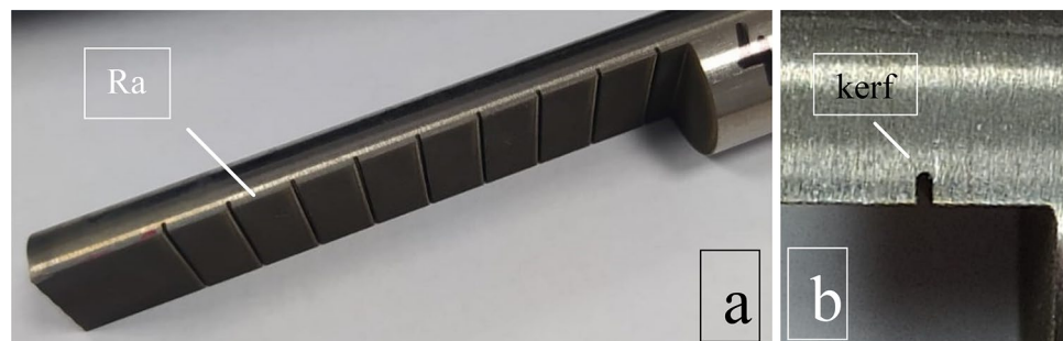
Figure 3. (a) Ra and (b) kerf images of this study.
