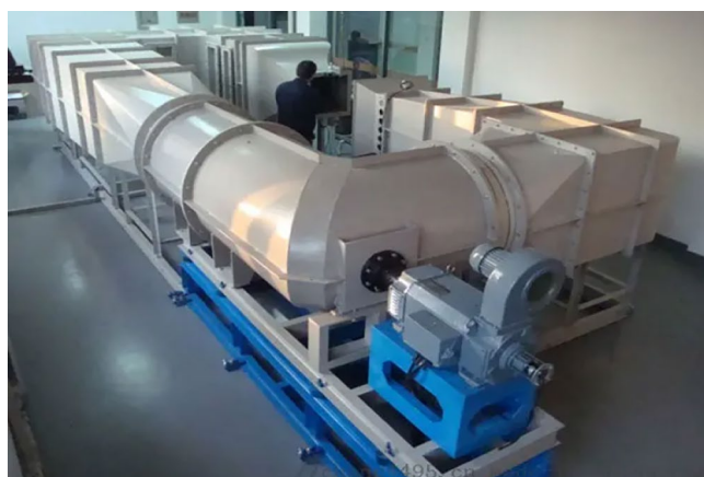
Figure 4. Circle closed low-speed wind tunnel.
