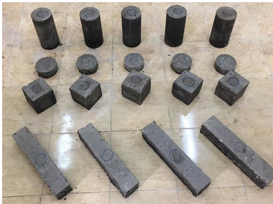
Figure 4. Concrete specimens for compressive, tensile, flexural, and impact strength.
