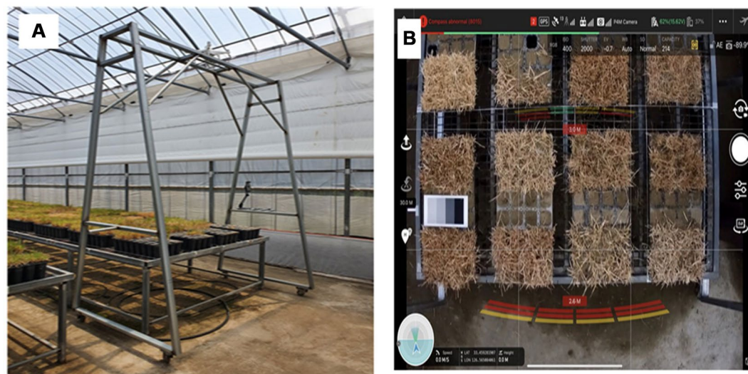
Figure 5. Customized vehicle for turf image acquisition (A) and captured DJI GS pro application image (B) where radiometric calibration target was located in.
