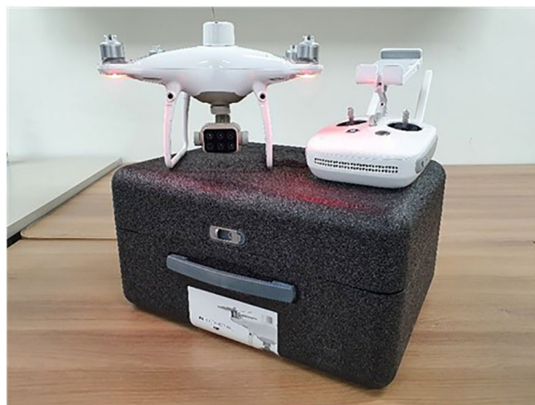
Figure 4. RGB camera sensor and multispectral sensor mounted Phantom 4 Multispectral.
