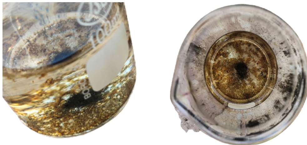
Figure 17. Formation of the iron cluster after dye degradation (MB).
