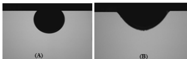
Figure 3. Images of contact angle change of an oil droplet on the sandstone surface solutions before (A) and after (B) wettability alteration aged by 0.01 M stearic acid and n-Heptane.
