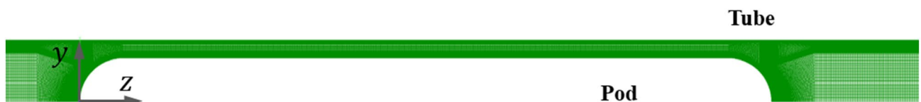
Figure 5. 2D half-model (ANSYS Fluent) of aerodynamic drag forces corresponding to its pod velocities at a BR of 0.6.
