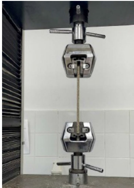
Figure 7. Tensile strength test setup (by authors).
