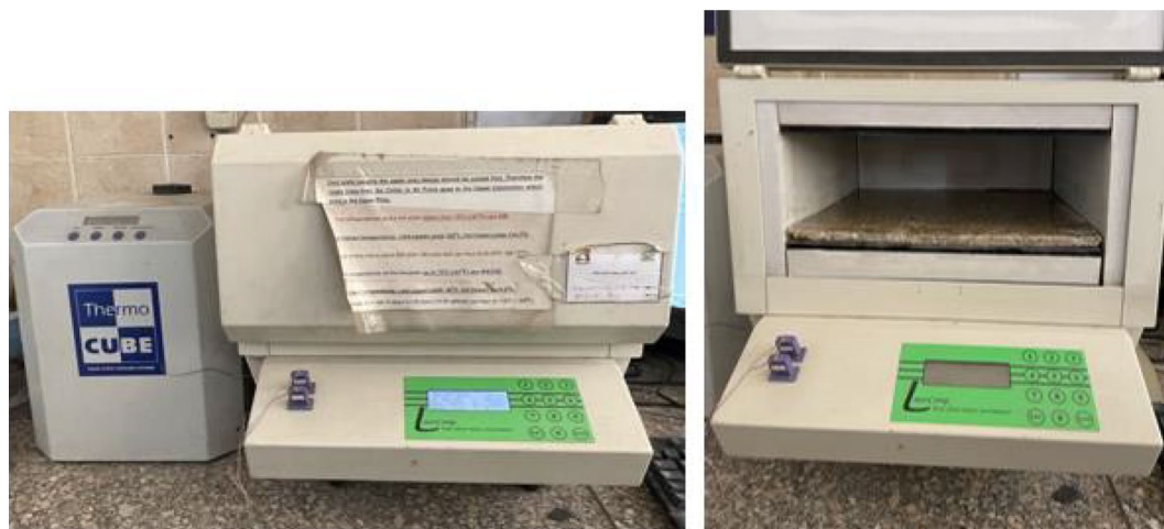
Figure 4. Thermal conductivity test using LaserComp Heat Flow meter (by authors).
