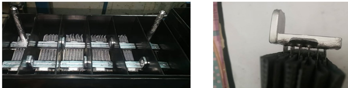
Figure 1. Lead-acid battery poles and strap. (Credits: German Co. for manufacturing batteries).
