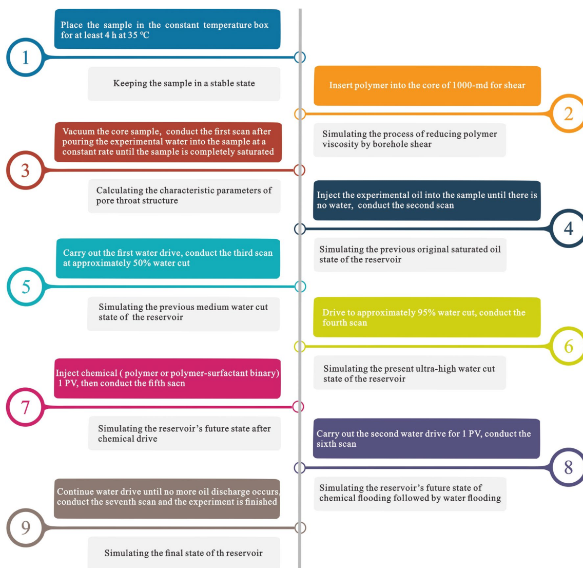
Figure 2. Flowchart of the NMR imaging displacement experiment.
