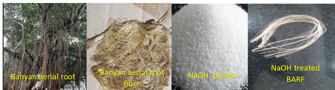
Figure 1. The extraction process of banyan aerial root fibre.
