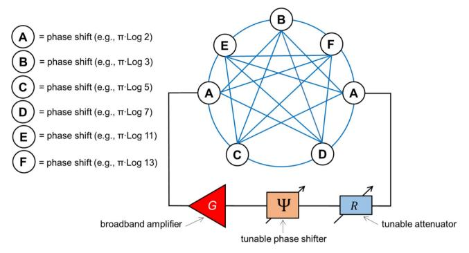
**Figure 4.** Schematics of the combinatorial device for TSP with six cities. There are two more phase shifters compared to Fig. 2 marked as E and F added to the mesh. These shifters provide  $\pi \times Log(11)$  and  $\pi \times Log(13)$  phase shifts, respectively.
