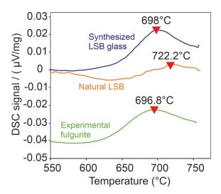
**Figure 6.** Simultaneous thermal analyses of the experimental fulgurite, synthesized LSB glass and natural LSB specimens (raw data). The revers triangles refers the estimated peak glass transition temperature for each sample.
