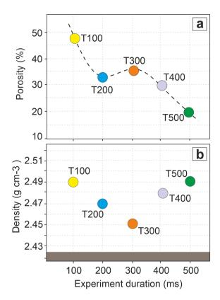
Figure 5. (a) The porosity calculation from 2D image analysis of all fulgurites. (b) Density measurements of LSB, synthesized LSB glass and all fulgurites. The brown area represents LSB  $(2.42\pm0.02 \text{ g/cm}^3)$  and synthesized LSB glass  $(2.42\pm0.004 \text{ g/cm}^3)$  densities for comparison. The error of the calculated and measured values for each experimental run is within the size of symbols.
