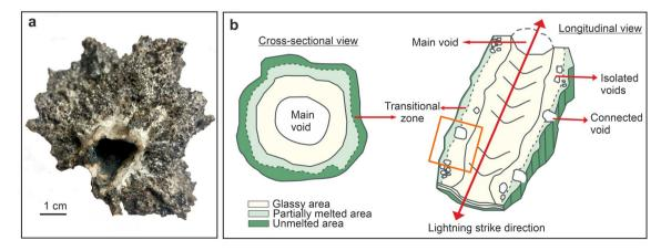
**Figure 1.** (a) An example of natural fulgurite (i.e., sand) from the Sahara Desert. (b) A representative cross-sectional and longitudinal views of a natural fulgurite with detailed morphological description. The orange square in the longitudinal view corresponds to the area where BSE images of the generated fulgurites in Fig. 4a–e are presented.
