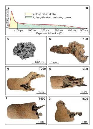
**Figure 3.** (a) Schematic composite electrical waveform of the experimental lightning components  $i_1$  and  $i_2$  for different experiment durations in  $\mu$ s and ms. (b). A SEM-BSE image of a pristine clast of the LSB. (c-g) Pictures of experimentally generated fulgurites under the variable long-duration continuing current (100–500 ms). The left end of each fulgurite corresponds to the portion adhering to the lower electrode in the experimental setup.
