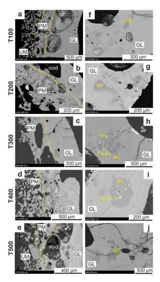
**Figure 4.** (a–e) BSE images of half face of each cut fulgurite as referred in Fig. 1b. Yellow dashed lines on the images mark the transitions between textural domains. (**f**–**j**) Images of the partially melted crystals in the glassy area of the fulgurites. *qtz* Quartz, *fds* Feldspar, *FeO* Iron-oxides, *GL* glassy area, *PM* partially melted area, *UM* unmelted area.
