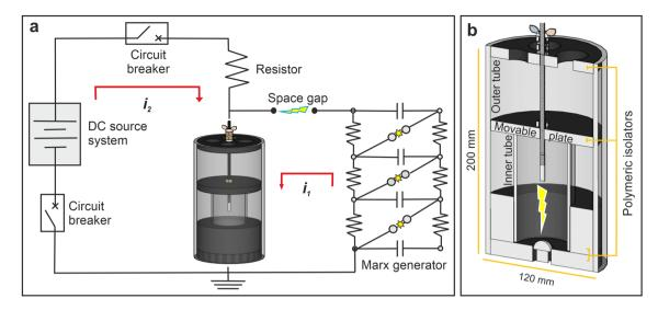
**Figure 2.** Schematic view of the experimental setup. (a) Circuit diagram of the DC source with trigger-pulse setup and 3D image of the sample container. The first return stroke ( $i_1$ ) indicates the lightning first return stroke component and the long-duration continuing current ( $i_2$ ) indicates the lightning continuous current component. (b) A sectional view of the cylindric sample container.
