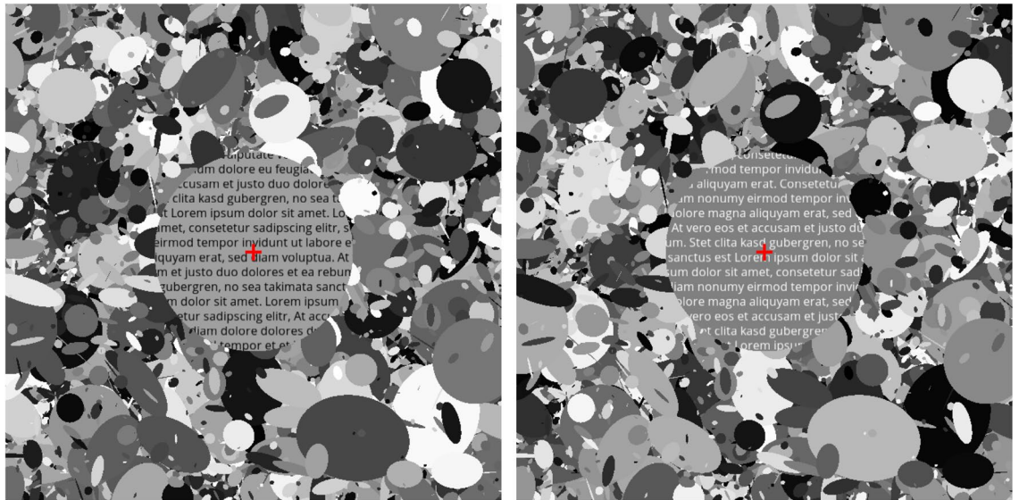
Figure 4. DLS with text component. Example for circle component of dark on bright (left) and bright on dark (right) text elements presented on a dead leaves stimulus [not to scale].
