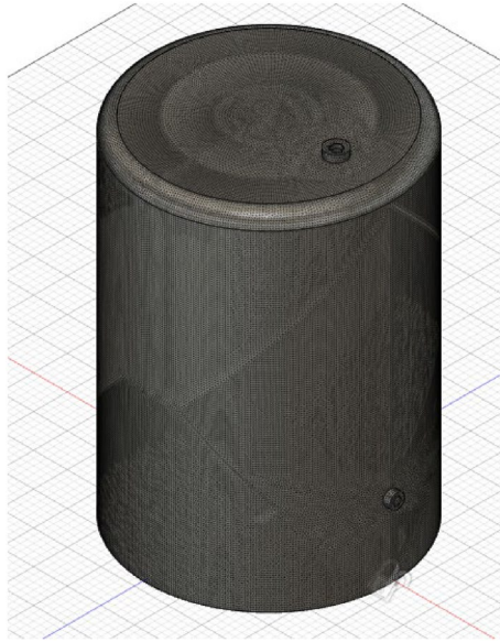
Figure 5. Meshing with element size of 30 mm.
