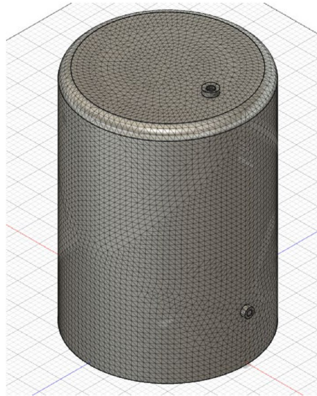
Figure 3. Meshing with element size of 100 mm.
