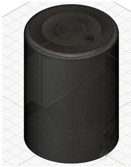
Figure 6. Meshing with element size of 20 mm.
