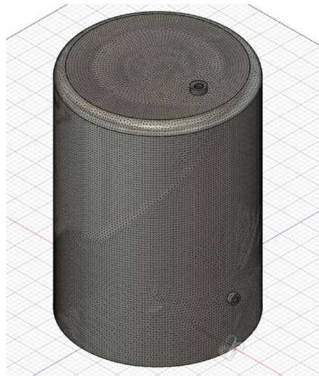
Figure 4. Meshing with element size of 50 mm.
