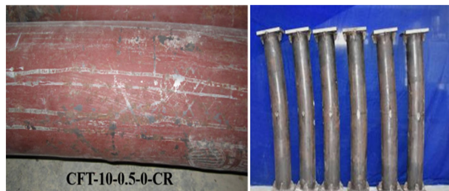
Figure 6. Failure mode for partial test specimens.
