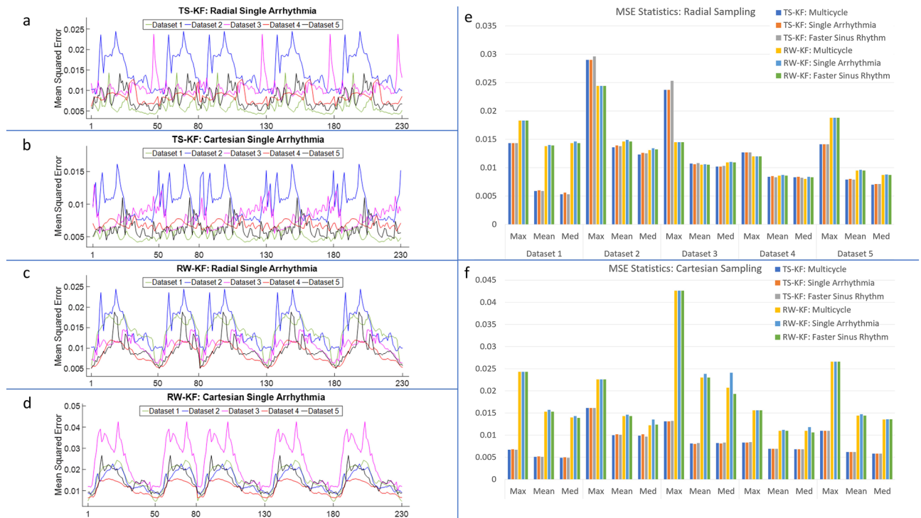
Figure 6. Mean-squared error (MSE) plots for the second primary scenario (single arrhythmic event), and MSE statistics for all scenarios. The subplots demonstrate the MSE for the second primary scenario across all UK Biobank datasets: (a) two-stage Kalman filter (TS-KF) with radial sampling, (b) TS-KF with cartesian sampling, (c) random-walk Kalman filter (RW-KF) with radial sampling, and (d) RW-KF with cartesian sampling. The x indices represent the frame number. Except for the index labeled “1”, each index also indicates the last phase of the corresponding cardiac cycle. (a–d) All demonstrate the robustness and consistency of our two-stage Kalman filter. Across all datasets, the MSE exhibited convergence. Subplot (e) demonstrates the maximum, mean, and median (med) values for all primary scenarios using radial sampling across all UK Biobank datasets. The MSE for the OCMR dataset is not available, as prospectively undersampling precludes the availability of the ground truth. Note that in general the TS-KF offered improved or comparable performance to the RW-KF. Subplot (f) demonstrates the maximum, mean, and median values for all primary scenarios using cartesian sampling across all datasets. Note that the TS-KF vastly outperforms the RW-KF for this sampling scheme.
