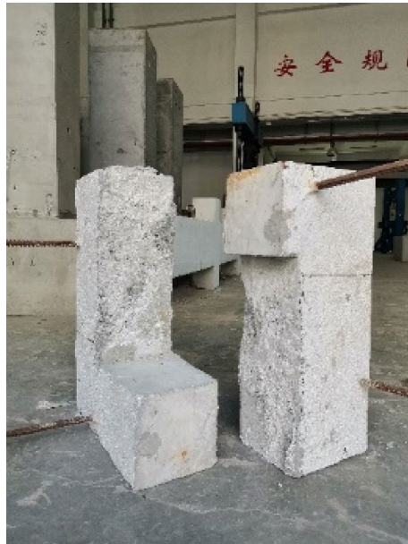
Figure 8. Failure mode of DS4.
