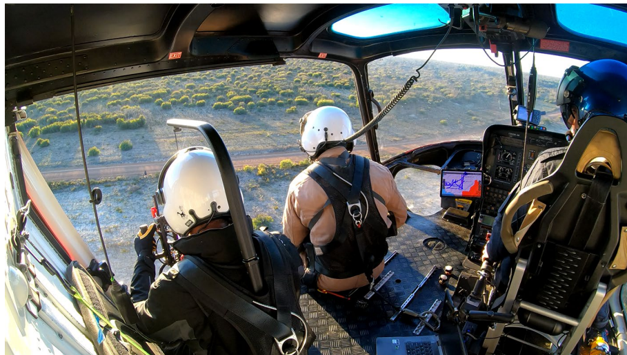
Figure 2. Crew configuration of thermal aerial culling in an AS350 B3 Squirrel helicopter. The pilot is in the front right, shooter in the front left, and thermal operator in the rear left. The shooter and the thermal operator are secured to the helicopter using approved aviation quick-release harnesses.
