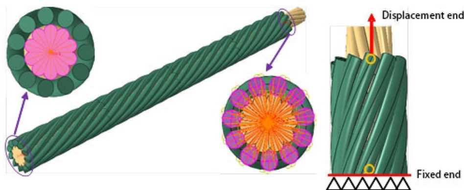
(a) Boundary condition constraint plot of the model. (b) Schematic of the model with applied loads.
