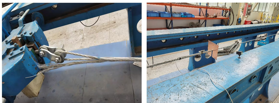
Figure 6. Preformed helical fitting test instruments and preformed armor rods.
