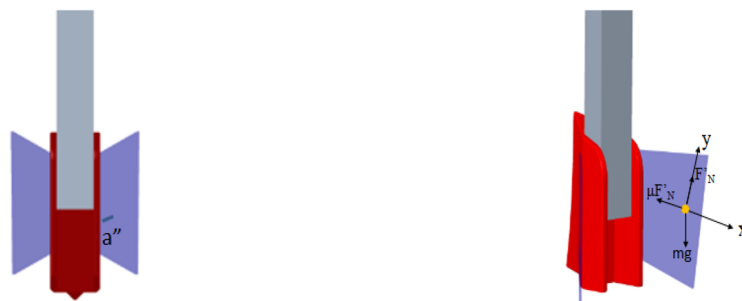
(a) Projection Angle of Rear Inclination Angle of Retaining Plate at Front Datum Plane (b) Stress analysis of the retaining plate in the soil during operation
