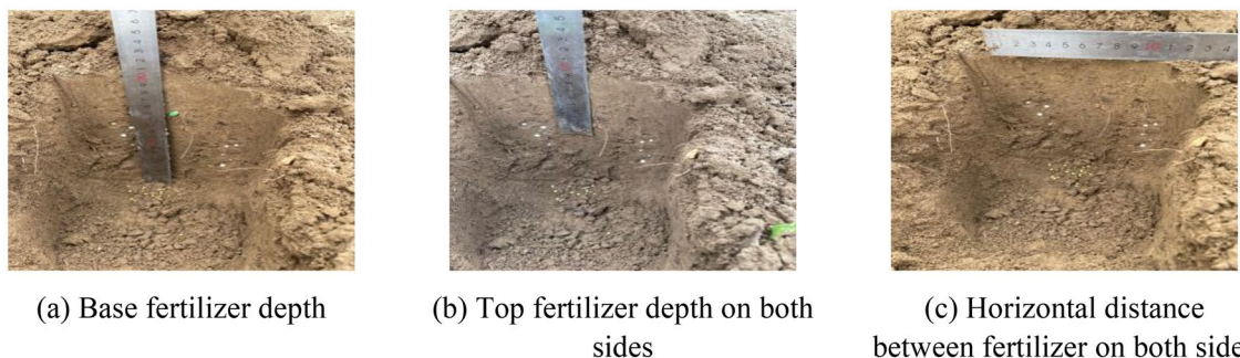
Figure 13. Fertilization effect diagram of U-shaped fertilization device.
