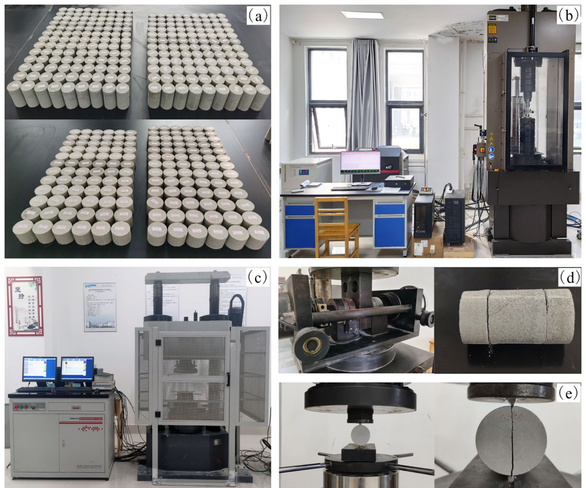
Figure 3. Mechanical parameter tests of samples. (a) Experimental samples; (b) MTS-815 rock mechanics testing machine; (c) YAW6206 computer-controlled electro-hydraulic servo pressure testing machine; and (d) direct shear test; (e) split test.
