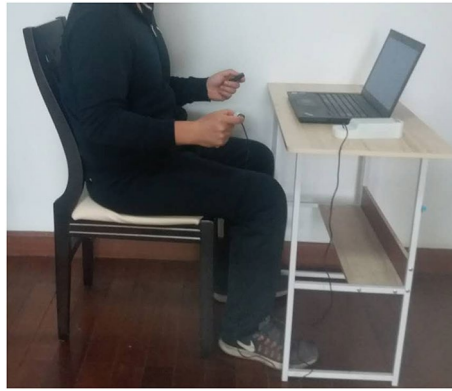
Figure 1. Standardized body and monitor positioning were used for the pinch force reproduction measurements.
