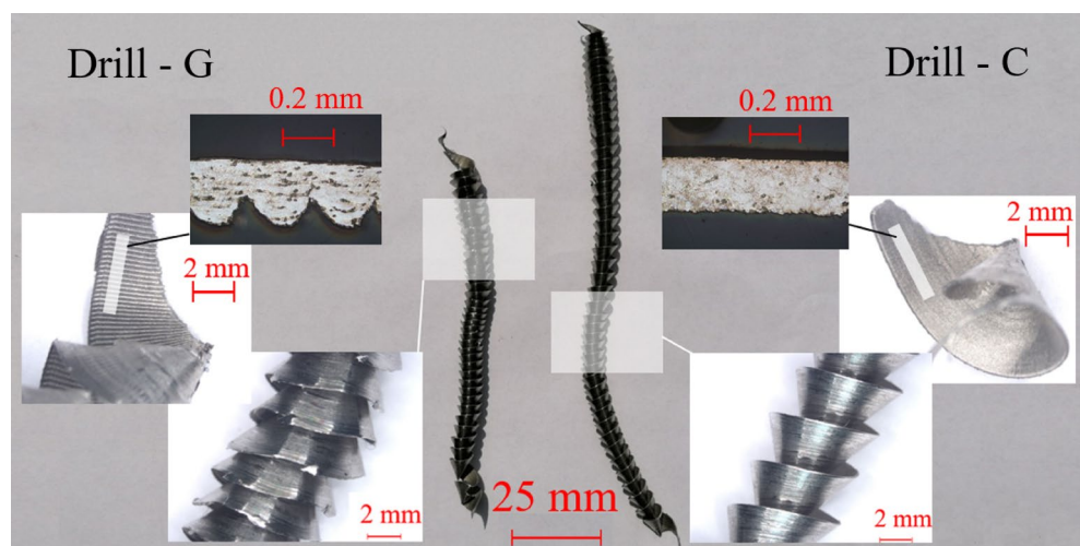
Figure 18. Comparison of the chip morphology formed by the stable drill C and the chips formed during the unstable drilling process by the tool G.
