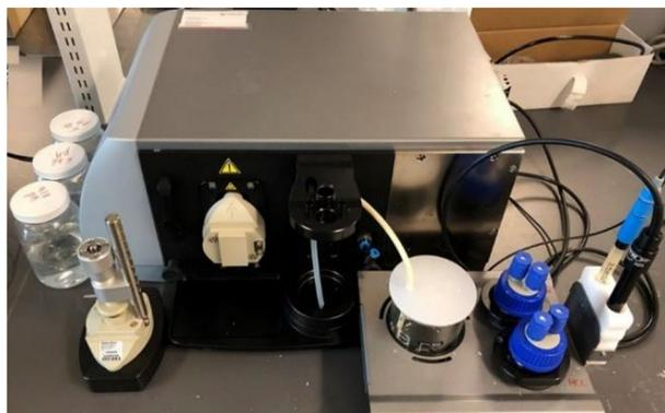
**Figure 2.** Schematic of the zeta potential measuring device and elements.
