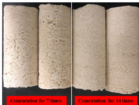
Figure 7. Typical microbial cemented coral sand samples under different cementation times.
