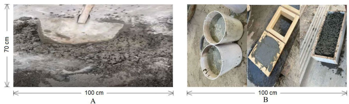
Figure 2. (a,b) Mixing of concrete (c–e) Moulds.
