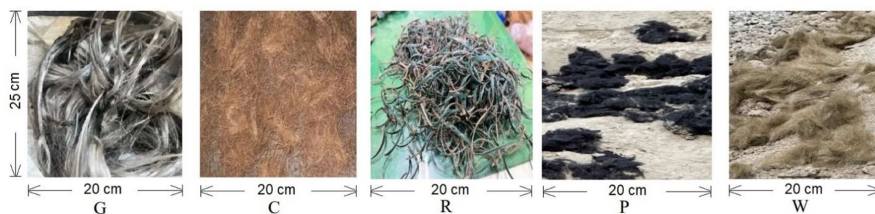
Figure 1. (G) Glass waste, (C) Coconut waste, (R) Rubber waste, (P) Polyester waste, (w) Rock wool waste.
