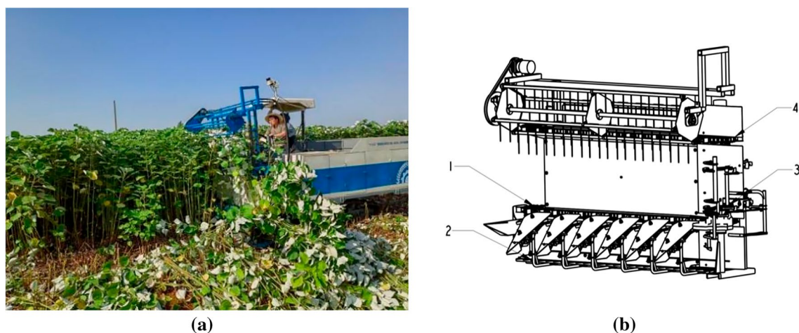
Figure 1. Ramie harvester. (a) Field harvest, (b) harvester structure. (1) Bottom chain, (2) cutter, (3) baling device, (4) second row chain.
